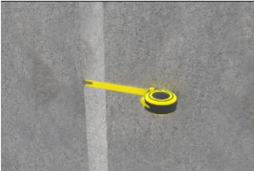
Ref 1 - Measure Gap opening every 5 to 7 feet (1.5 to 2.1 M).
